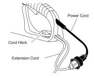
Figure 9 - Looping Extension Cord over Cord Hitch
